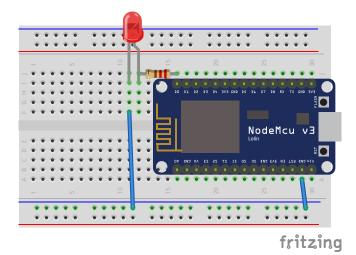
The colors on the wires used does not matter. The resistors orientation is not important, but the LED's orientation is important.
