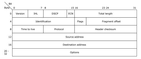
Note that the "total length" field is 16 bits, 2 bytes, it's maximum value is 64k, 65536.
