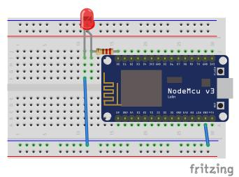
The colors on the wires used does not matter. The resistors orientation is not important, but the LED's orientation is important.
